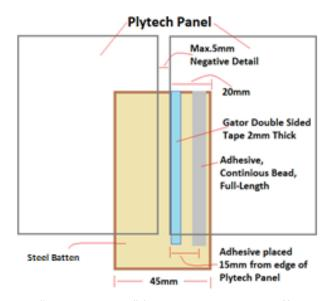
batten along all edges that will have the "negative detail" (as you will not have sufficient space for both the adhesive and tape).
